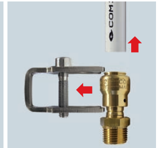
3 With the clamping fixture held in this position the pipe can be removed. The fitting can be used again without the need for replacement parts
